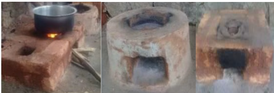
Photo 1: Examples of energy saving stoves (Majiko Banifu)
