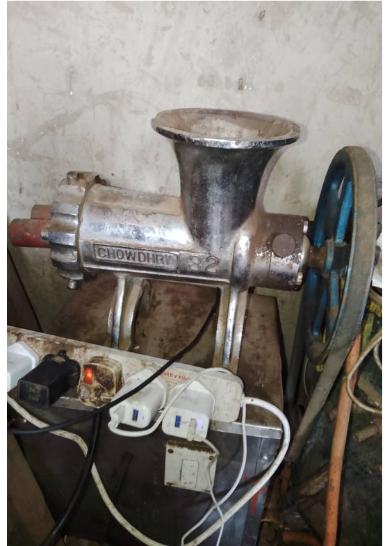
Photo 5: Alternative Charcoal making machine
